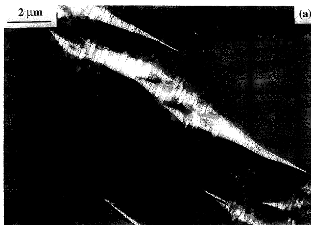
Figure 1 Crazing in a 0.3\ \mu\text{m} thick solution cast unmodified PMMA film
