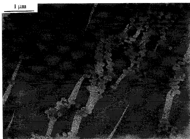
Figure 2 Deformation in a 0.15\ \mu\text{m} thick solution cast film containing two-layer particles (note the tendency for the particles to agglomerate)
